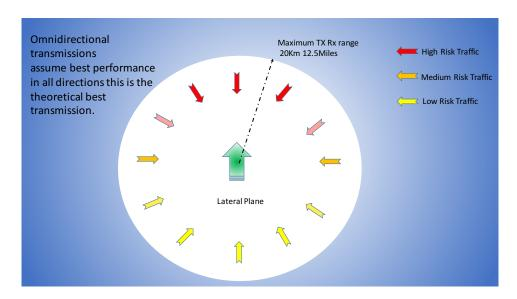
Therefore, when positioning your antenna you should take the probability of the position of other aircraft into account along with the metal and water content of your aircraft that will be in the way of your omnidirectional transmissions.
